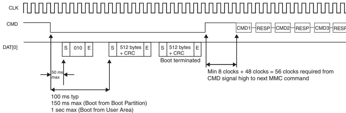
**Figure 5.2** MultiMediaCard State Diagram (Alternative Boot Mode)
