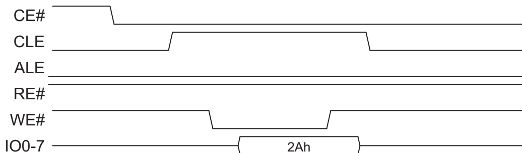
Figure 5.3 Volatile Lock All Blocks Operation Sequence
